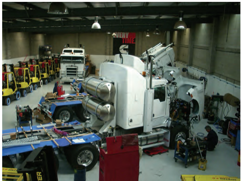
Mitchell Corp Pty Ltd trucks being converted to Dual-Fuel™ in Melbourne, Australia
